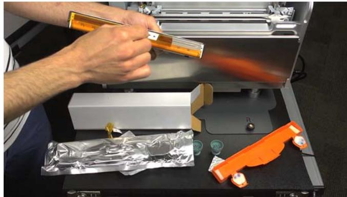
**Caution:** Dispose of the removed strips immediately and do not allow the removed strips to touch the electrical contacts or printhead nozzles.
