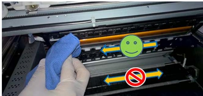
**Note:** Wiping should always be just a single move from one end to the other. Never wipe back and forth as that would transfer some waste ink back to the printhead nozzles contaminating the colors.
