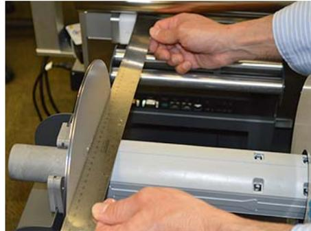
Adjust the unwinder position as needed. Then tighten the thumbscrews on the unwinder base plate.
