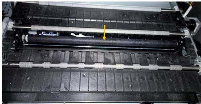
The wiper roller comes up and it is rotating slowly. Visually inspect the wiper roller. Remove any particles that might be stuck on the roller and could damage the printhead nozzles. Look for any visual damage on the roll and verify that surface of the MFR is “fluffy” still. In case the surface of the roller is shiny, then replacement of the MFR is recommended.
