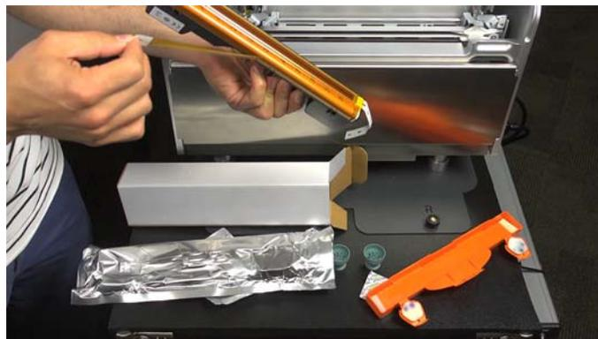
Grasp the pull tab and slowly peel back the plastic strip covering the printhead nozzles. Maintain an angle of no less than 45 degrees with the printhead surface when pulling on the strip.
