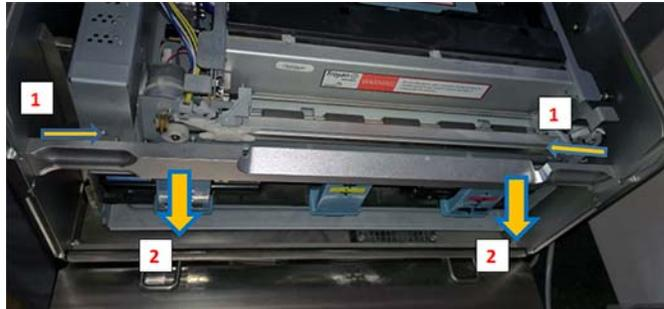
The crossbar is fixed by 2 latches on the inner side of the bar. Pull both latches towards the middle (1) and pull out the cross bar (2).
