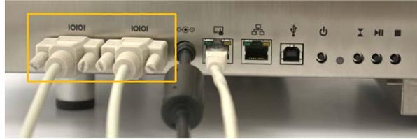
The order of the serial ports does not matter. Both Unwinder and Rewinder can be connected to either the first or the second serial port. The QL-240 printer automatically detects and identifies the winders.
