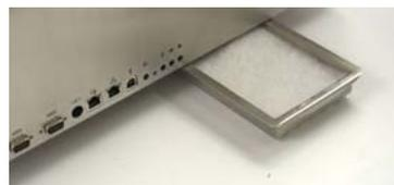
Both filters are consumables and can be ordered as a spare part. Part numbers are 20020011 for the aerosol filter and 20020012 for the dust filter.
