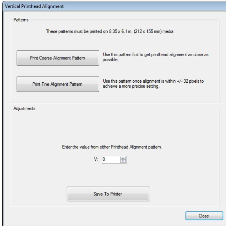
This window provides a coarse and fine alignment pattern. Start with the coarse adjustment and align the printheads as close as possible. Then use the fine adjustment for precision alignment.
