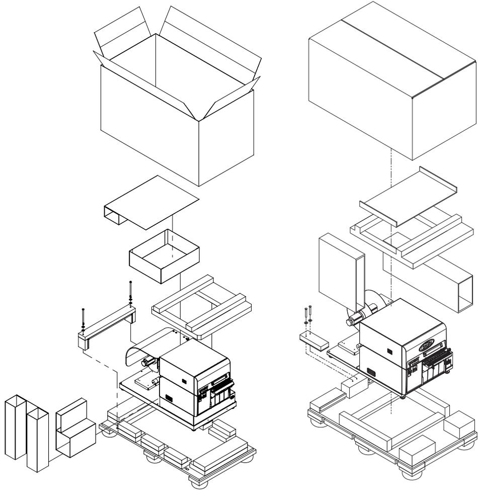
**Note:** The printer model on the left has the roll cover. The printer model on the right does not have the roll cover.
