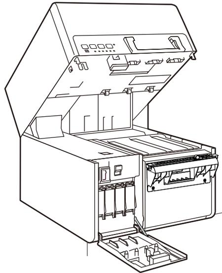
**Note:** Never attempt to open the upper unit by force or hit the door. This could damage the printer or result in poor print quality. Always open and close the upper unit slowly.
