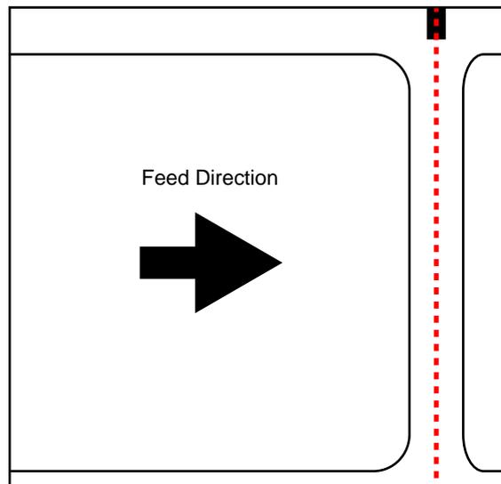
If the cut is not located in the center of the reflective mark, label feeding errors may occur. Adjust the stop position so the cut is centered on the mark. Setting the Stop Position
