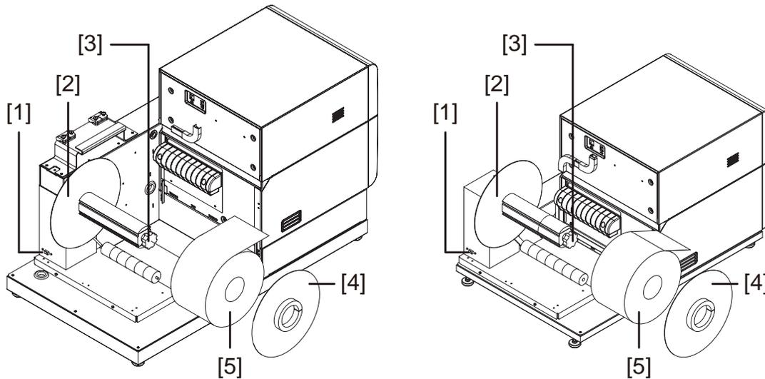
**Note:** The printer model on the left has the roll cover (not illustrated). The printer model on the right does not have the roll cover.
