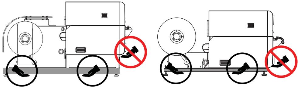
**Note:** The printer can weigh up to 170 pounds (77 kilograms). Three persons are required to lift the printer. Lift only by the black frame on the bottom of the printer. Do not grasp any other part of the printer to lift it. Do not lift the unit by the print engine. Attempting to lift the printer in an improper position can result in fall of the printer or injury.
