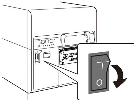
**Note:** Never turn off the main power switch during a print job. This could cause damage because the printhead cannot return to the home position.
