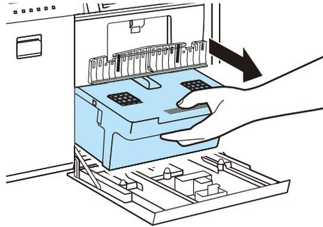
When removing the maintenance cartridge full of ink, take care not to incline or drop it. The spilled or scattered ink may stain the floor or clothing.
