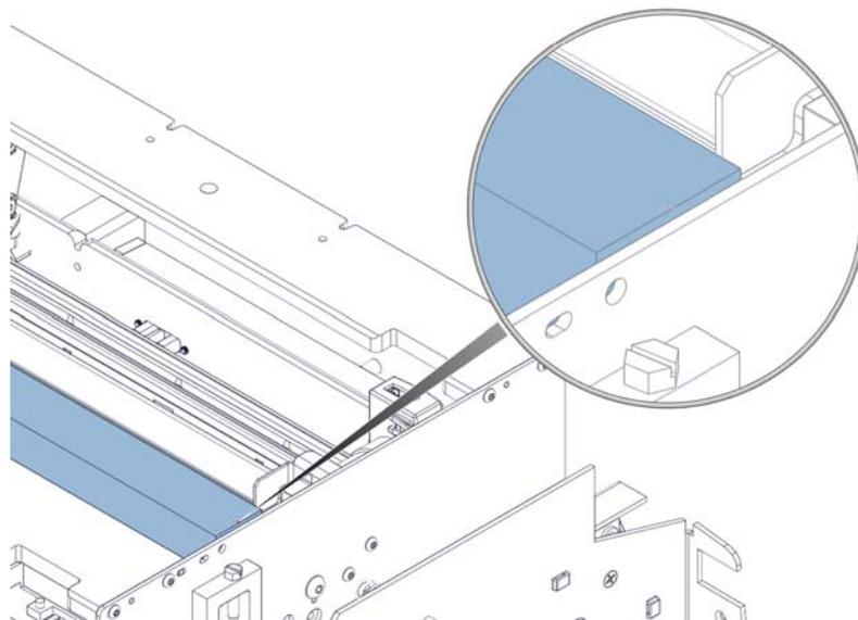
If either side is not level, follow the rest of this procedure for angularity adjustment instructions.
