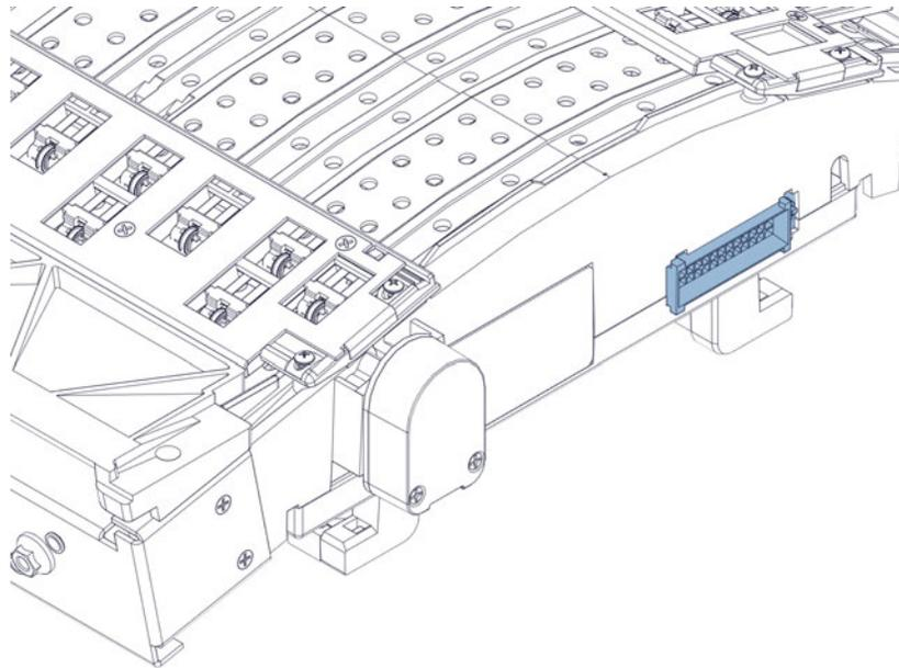
The mating connector inside the printer is illustrated below.
