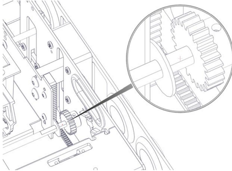
Lift or lower the printhead lift by the height of one gear tooth. Then slide the gear inward to engage it with the printhead lift teeth. Do not pinch the nylon washer. The nylon washer should be able to spin freely.
