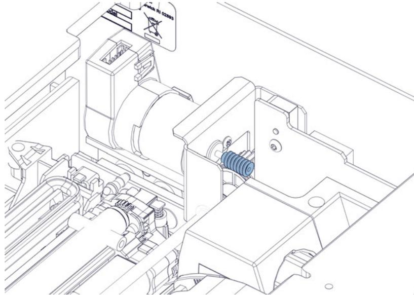
When the set screw is facing upward, it will be accessible during the rest of this procedure.
