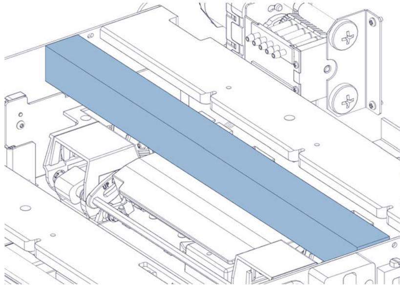
TF1262 will be used to test for angularity on each side of the bracket with respect to the print engine left/right plates.
