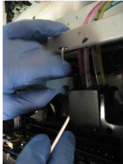
The second side should easily slide out of the hinge.
